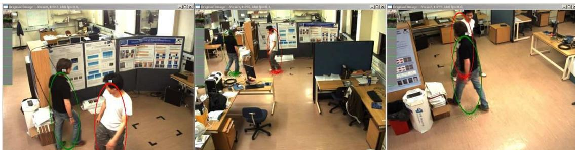
Figure 9: The ellipses show estimated positions projected on each view and panel on top-left are texture images of the subjects.
