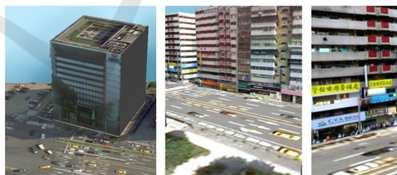
Figure 1: Examples of the reconstructed building models, which are textured with building elevation images automatically extracted from the panoramic images to provide the realistic impression.
