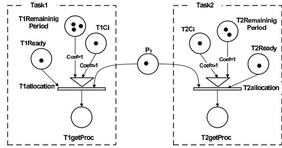
Figure 4: Allocation processor.
