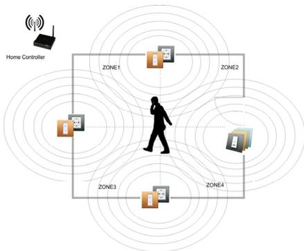
Figure 1: Presence detection in smart energy ecosystem.
