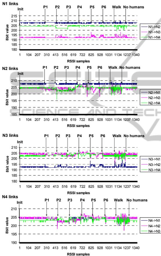
Figure 6: Experimental results for alu/plastic walls.
