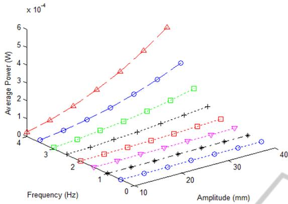
Figure 8: Simulated average power harvested from the TEEH transducer.
