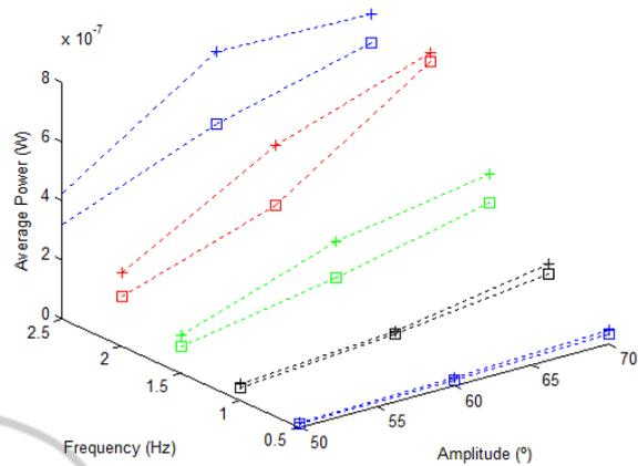
Figure 10: Experimental average power harvested from the REEH transducer (the plus sign refers to peak-to-peak amplitudes in the range -10 mm to 60 mm, -10 mm to 50 mm and -10 mm to 40 mm; the square refers to peak-to-peak amplitudes in the range -20 mm to 50 mm, -20 mm to 40 mm and -20 mm to 30 mm).
