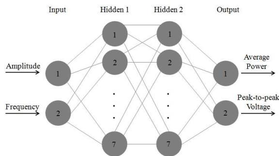
Figure 6: Architecture of the ANN used in modelling for the average power and peak-to-peak voltage of the PEH transducer.
