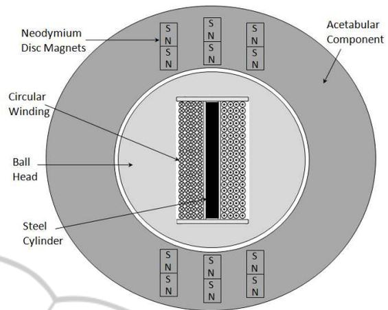
Figure 4: Scheme of the REEH transducer.
