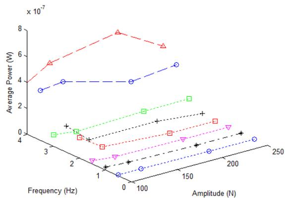
Figure 14: Experimental average power harvested from the PEH transducer.
