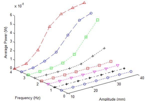
Figure 7: Experimental average power harvested from the TEEH transducer.
