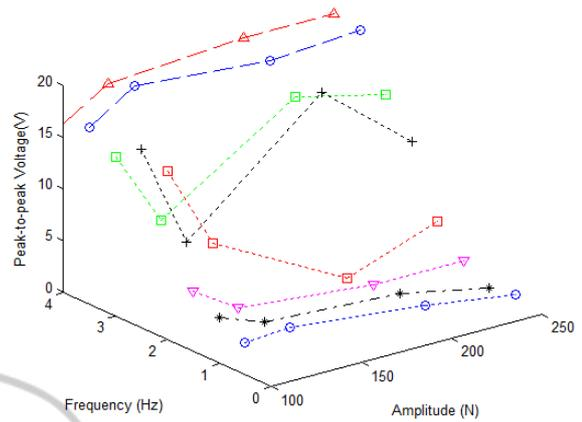
Figure 15: Experimental voltage harvested from the PEH transducer.
