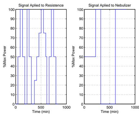
Figure 4: Signals applied to nebulizer and warm resistance.
