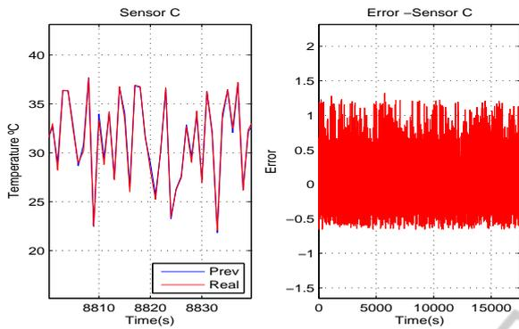
Figure 6: Comparisons, and error, between MLP outputs and the training data of temperature (worst case).
