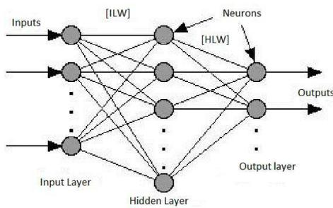
Figure 3: Multilayer perceptron network architecture, (Haykin, 2008) adapted.
