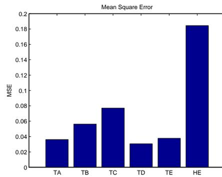
Figure 8: The mean squared error (MSE) between the signals of network and real signals for each sensor (validation set).
