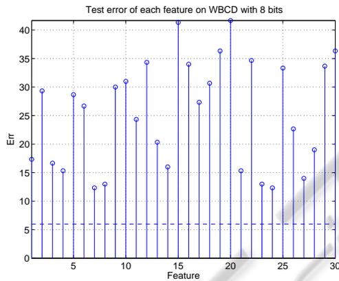
Figure 2: Test set error rate of naïve Bayes using only a single feature, discretized with  $q = 8$  bit by the U-LBG2 algorithm, on the WBCD dataset. The horizontal dashed line is the test set error rate obtained with the full set of  $p=30$  features.
