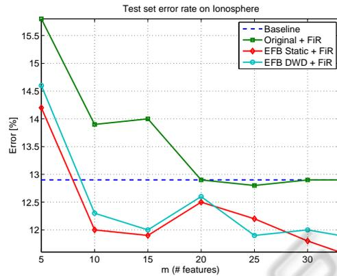
Figure 8: Test set error rate (average of ten runs, with different training/test partitions), as functions of the number of features, for the naïve Bayes classifier, using FS by the FiR method, for the Ionosphere dataset on original, static, and dynamically discretized features.
