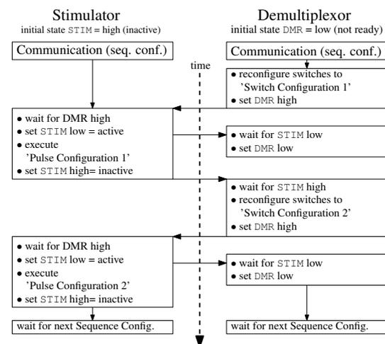
Figure 3: Execution of a sequence where two stimulation pulses are generated and distributed over different switch configurations.
