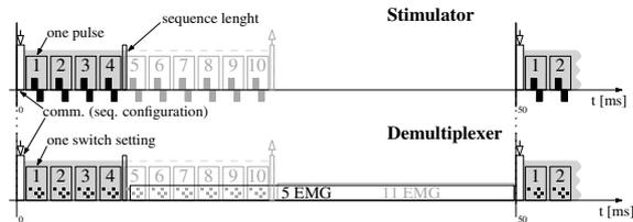
Figure 1: Example for a sequence of 4 pulses for the stimulator device and one demultiplexer. The largest possible sequence is indicated in gray.
