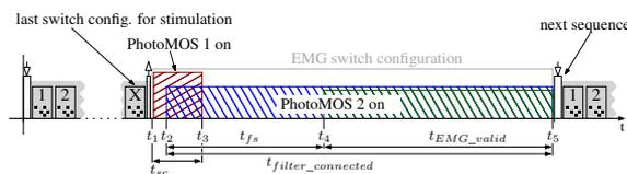
Figure 4: EMG protection and discharging timing,  $t_1 \dots t_4$  depend on sequence length and array setting.
