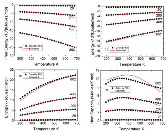
Figure 3: Comparison of (a) free energy, (b) mean energy, (c) entropy, and (d) heat capacity estimates. Exact values are calculated by matrix multiplication scheme, estimated values are calculated by fundamental relation. The lengths of chains are shown on each curve.
