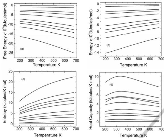
Figure 2: (a) The free energy as a function of temperature,  $T$ , for different length proteins. (b) energy as a function of  $T$ . (c) entropy as a function of  $T$ . (d) heat capacity as a function of  $T$ . The curves in parts (a),(b), and (c) are ordered from top to bottom represent proteins with the following numbers of residues: 10, 40, 120, 160, 226, 349, 408, 456, 545, and 802, respectively. In part (d) they are in reverse order.
