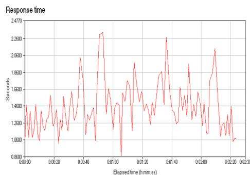
Figure 5: FTP-get response time for Carrier 1 at junction of Trans Canada 16/Hwy 216 (point B).
