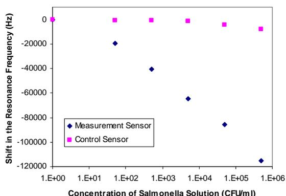
Figure 8: Response of 500  $\mu\text{m}$  long biosensor exposed to increasingly higher concentrations of *S. Typhimurium*. The detection limit is less than 50 CFU/mL. The response of the control sensor (devoid of phage) is also shown.
