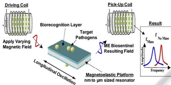
Figure 2: Detection principle of a magnetoelastic (ME) biosentinel. A driving coil generates a modulated magnetic field that drives the ME resonator into vibrational resonance. Binding of the target bacteria to the bio-molecular recognition layer immobilized onto the resonator increases the mass of the sensor resulting in a decrease in resonant frequency.
