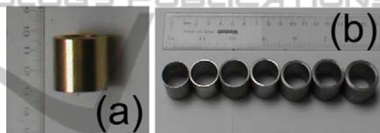
Figure 4: The gold-plated N52 grade neodymium-iron-boron ring (a) and stainless steel rings of various thicknesses (b) which were used in subsequent testing.
