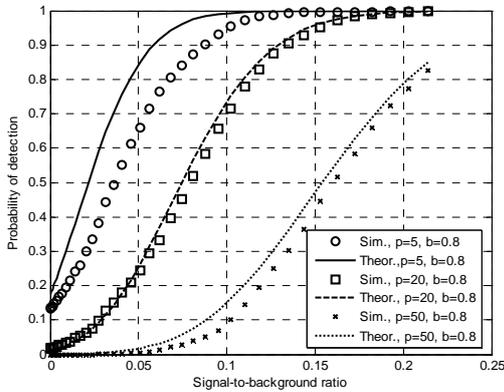
Figure 1: Probability of detection versus  $SBR_{in}$  for proposed system for target fill factor  $b = 0.8$ . The lines depict the analytical results, whereas the markers show Monte Carlo simulation trial results. The false alarm rate  $F=10^{-3}$ , number of measurements  $N=200$ , 3 targets with subspace dimensions:  $p=5, 20, 50$ , uncorrelated background  $\rho=0$ ;  $A=1$ .
