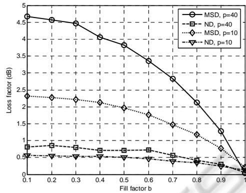
Figure 3: Loss factor of detection versus fill factor of target  $b$  for proposed system (ND) and well known (MSD). 2 targets with dimensions:  $p = 10$  and 40. Simulation results for  $F=10^{-3}$ , number of measurements  $N=200$ , uncorrelated background;  $A=1$ .
