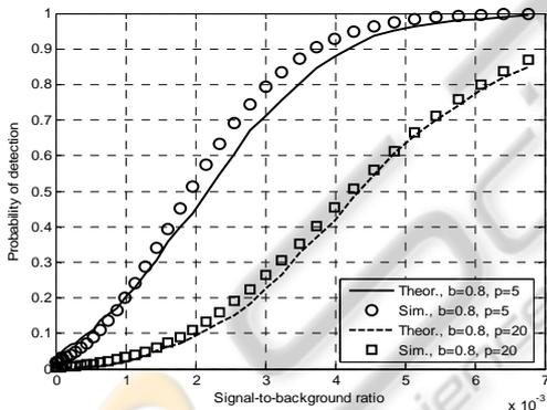
Figure 2: Probability of detection versus  $SBR_{in}$  for proposed system for target fill factor  $b = 0.8$ . The lines depict the analytical results, whereas the markers show Monte Carlo simulation trial results. The false alarm rate  $F=10^{-3}$ , number of measurements  $N=200$ , 2 targets with subspace dimensions:  $p=5$  and 20, correlated background  $\rho=0.9$ ;  $A=1$ .
