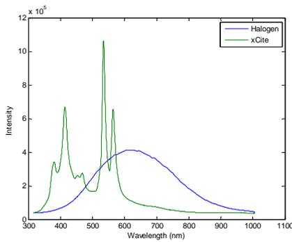
Figure 2: System response to white standard for tungsten halogen and xCite light sources.
