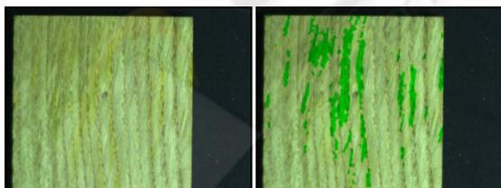
Figure 1: Example of yellow stained wood (left) the results of our classifier (right). For display we have lit the sample with fluorescent light which makes the yellow stain more apparent than under tungsten halogen light.
