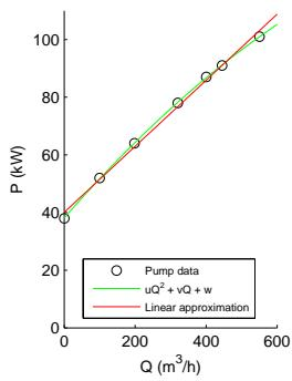
Figure 1: Fitted power function using pump data.
