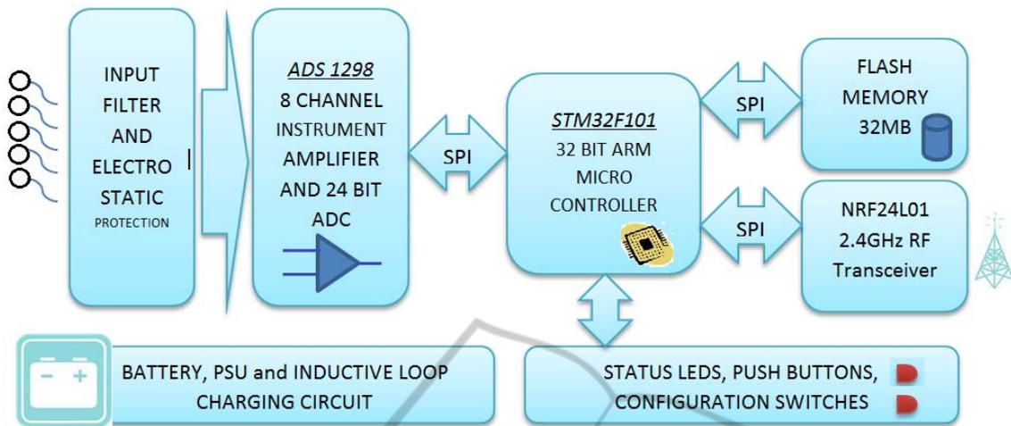
Figure 1: EEG Sensor, primary hardware components.
