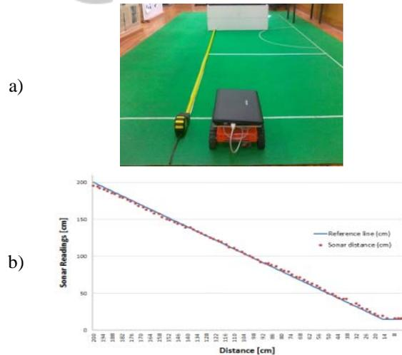
Figure 4: a) Experimental scenario. b) Range testing results.
