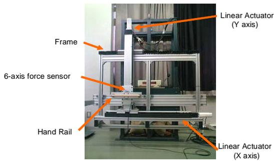
Figure 1: A handrail that could give assistance to users in standing.
