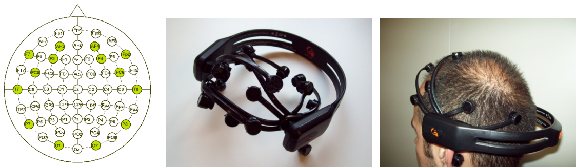
Figure 1: Sensor placement of the 14 data channels in the Emotiv Epoc, according to the 10/20 International System (left). Emotiv Epoc (centre). User with the Emotiv Epoc (right).
