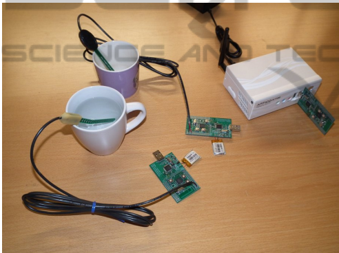
Figure 2: Two Active Tags with moisture sensors and the RIBS PC with Gateway.
