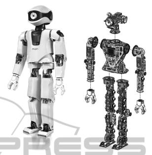
Figure 2: The modular humanoid robot MYON. Left: Image of the functional robot including the exoskeleton shells. Right: Overview of the robot's detachable body parts.
