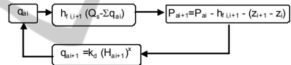
Figure 2: Iterative computation of pressure (Pai, kPa) and discharge (qai, ls<sup>-1</sup>) for each outlet i.
