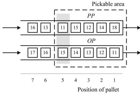
Figure 3: An example of the content of product ( $PP$ ) and order ( $OP$ ) buffers. The numbers represent the IDs of pallets. A product pallet at  $PP$  belongs to an order pallet at  $OP$  with the same ID. The robot is currently at position 5.
