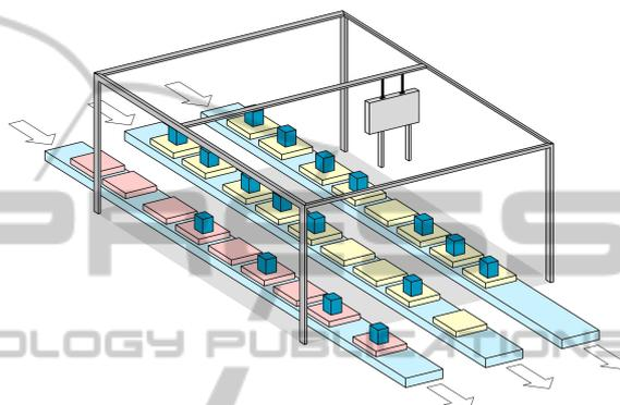
Figure 1: Layout of the automated order-picking workstation. One buffer lane is used for order pallets (red) and two buffer lanes are used for product pallets (yellow). The pickable area is the area inside the frame. The arrows denote the direction of pallets movements.
