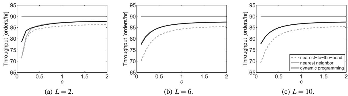
Figure 9: Order throughput for variable pickable area size  $L$ ,  $p = 0.8$ ,  $k = 10$ ,  $N = 30$ .
