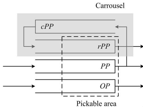
Figure 2: Conceptual design of the automated order-picking workstation.
