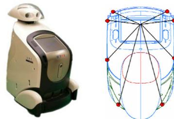
Figure 4: Robot platform and arrangement of microphone.
