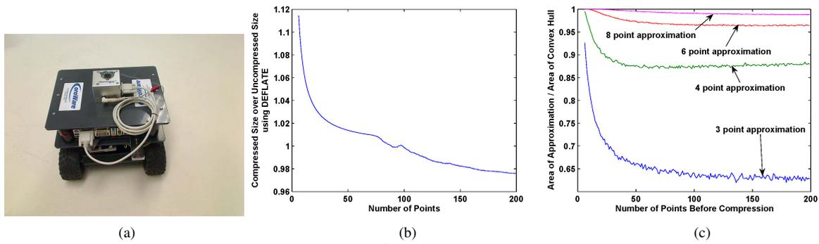
Figure 4: (a) Photograph of a Corobot fitted with a Stargazer localization device. (b) Compression ratio obtained using the DEFLATE zip library. (c) Ratio of the area of the approximated polygon calculated using the min- $\epsilon$  algorithm and the area of the convex hull for different sizes ( $m = 3, 4, 6$  and  $8$  vertices) of the compressed set.
