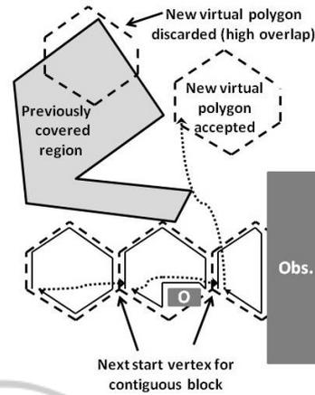
Figure 3: Path of a robot showing the definition and coverage of contiguous blocks. When contiguous block definition fails due to the obstacle on the right-end of the diagram, the robot iteratively selects a new virtual polygon whose percentage overlap with previously covered regions falls below a certain threshold.
