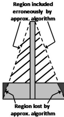
Figure 2: Effect of vertex compression of two overlapping rectangles with a combined polygon with  $m = 4$ . The gray area (light and dark) is the *desiredArea*, the stroked area is the *gainedArea* and the dark gray area is the *lostArea*.
