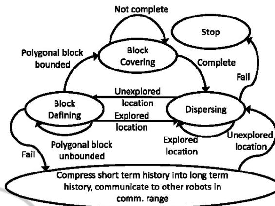
Figure 1: State transition diagram for a robot's behaviors.
