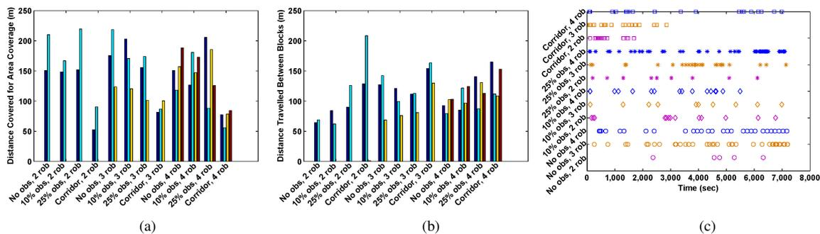
Figure 6: Distances traveled (m) by each robot (a) while covering the environment and (b) while not covering the environment (overhead) under the different robot and environment configurations. (c) Frequency of communication between robots in the different scenarios.
