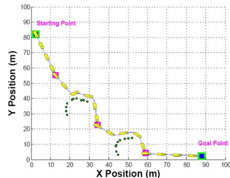
Figure 9: 2D Obstacle avoidance of AUV with circular obstacles of same size.
