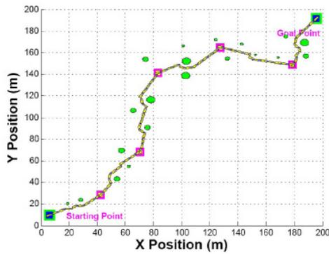
Figure 10: 2D Obstacle avoidance of AUV with circular obstacles of various sizes.
