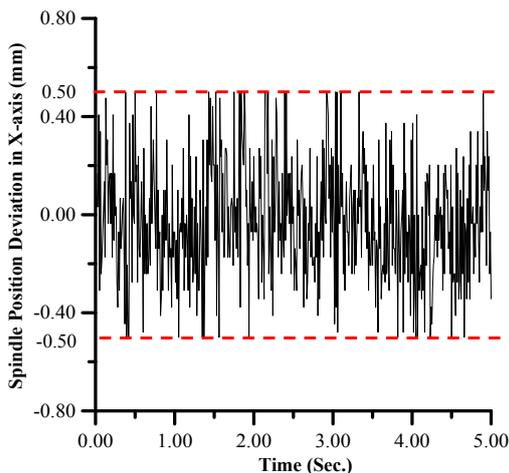
Figure 9: Spindle Position Deviation w/o AW Compensation (Speed: 6000RPM).
