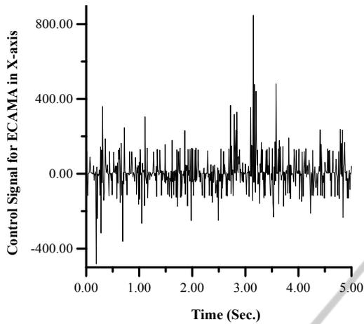
Figure 7: Controller Output w/o AW Compensation (Speed: 6000RPM).
