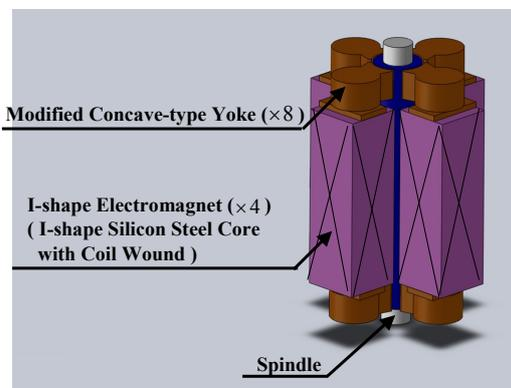
Figure 3: Configuration of ECAMA.
