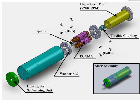
Figure 2: ECAMA and Spindle for Mill Machine.
