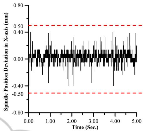
Figure 10: Spindle Position Deviation with AW Compensation (Speed: 6000RPM).
