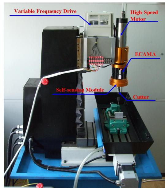
Figure 6: Test Rig for AW Compensation.
