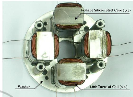
Figure 4: Prototype of I-shape Electromagnets (Bottom View).
