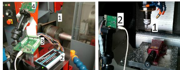
Figure 1: Left: assembly prepared to proceed with the first test for 64x64 retina. The components are 1. Lathe, 2. Logic Analyzer, 3. Sequencer Monitor AER and 4. 64x64 pixel retina, right: assembly prepared to proceed with the first test for 128x128 retina. The components are 1. CNC Machine and 2. 128x128 pixel retina.
