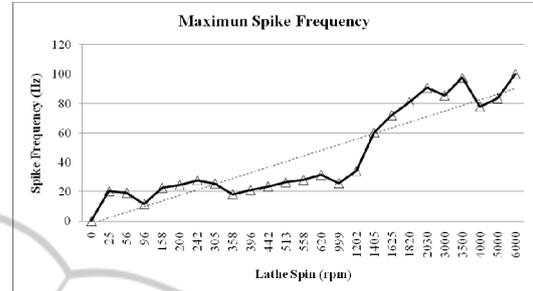
Figure 2: Maximum spike frequency evolution for the 64x64 retina spike frequency in front of the spin of the lathe expressed at rpm.
