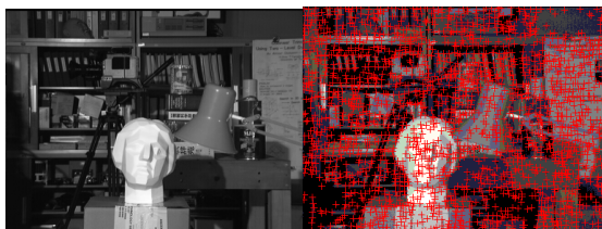
Figure 5: Edge detections in a features-based algorithm.
