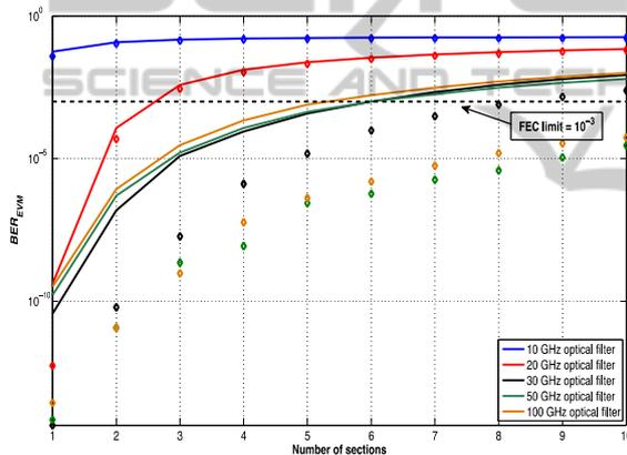
Figure 7:  $BER_{EVM}$  as a function of the number of sections used in the optical link obtained for an OSNR of 25 dB (diamonds) and 20 dB (continuous lines) for different receiver optical filter bandwidths. The error probability corresponding to the FEC limit is also depicted.
