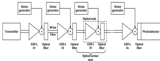
Figure 6: OFDM transmission system with several spans. Each span is composed by a fiber followed by the optical node constitute by an EDFA and an optical filter.
