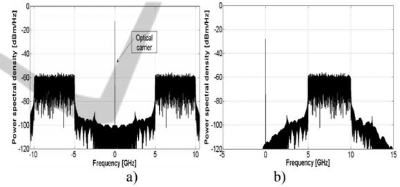
Figure 3: Power spectral density of the OFDM signal. a) DSB signal at the modulator output. b) SSB signal after filtering for a CSPR of 0 dB.
