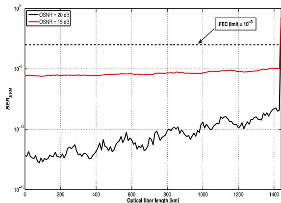
Figure 8:  $BER_{EVM}$  as a function of the optical fiber length in the optical link. The error probability corresponding to the FEC limit is also depicted.
