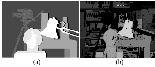
Figure 4: (a) Real depth of Tsukuba images. In black, the occluded parts. (b) The computed depth map. In black, unmatched regions and occluded parts.
