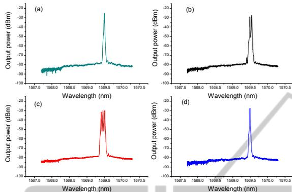
Figure 5: Wavelength switching of the fiber laser by adjusting the PC1, pump power of 134mW.
