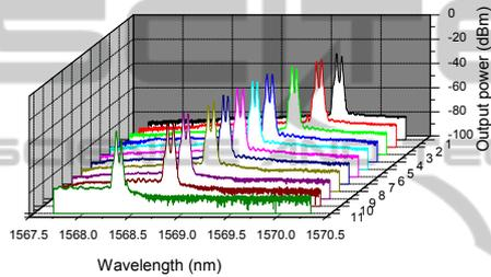
Figure 3: Experimental emitting spectra of the Erbium-doped fiber laser by tuning the reflection peak of the FBG.
