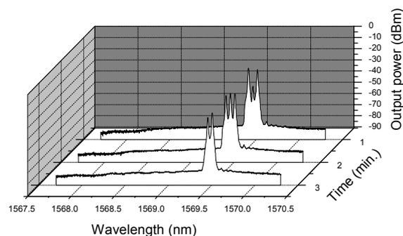
Figure 7: Measured output spectrum at three-wavelength lasing of 1569.408, 1568.460nm and 1569.512nm every 1minute for 3 minutes, pump power of 134mW.
