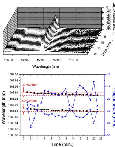
Figure 4: Measured output spectrum at fixed wavelengths of 1568.889 and 1568.944nm at 21-time repeated scanning spectra with a time interval of 1 minute, pump power of 134mW.
