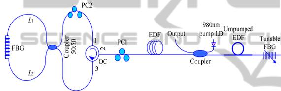
Figure 1: Schematic diagram of the proposed tunable and switchable Erbium-doped fiber laser with a simple linear cavity.
