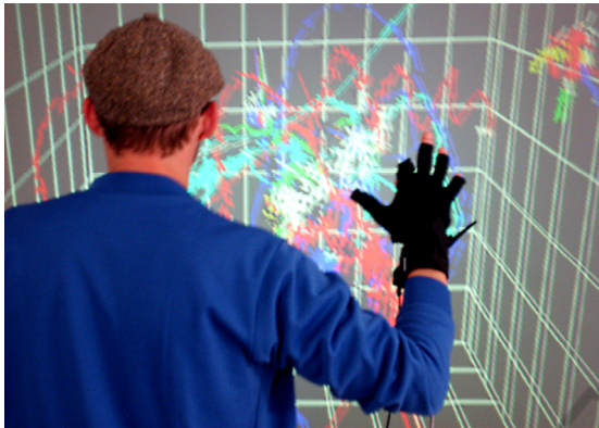
Figure 3: A user performing 3D graphical artworks using the 5dt glove-based interaction technique.
