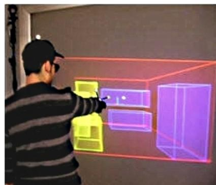
Figure 1: User manipulating the 3D objects using the human-scale VR platform.
