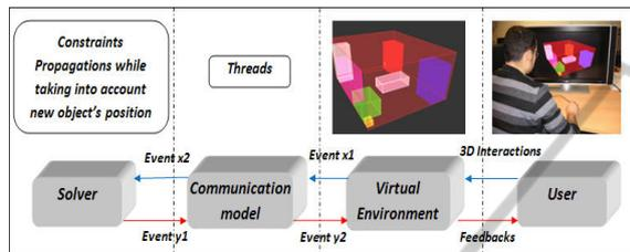
Figure 2: Illustration of the system architecture.
