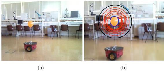
Figure 5: Real time target tracking. Left: experimental setup; right: target identification, where the initial guess for the target contour is presented in black, its temporal evolution is presented in red, and the final contour estimate is presented in blue.
