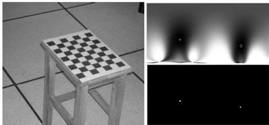
Figure 3: Illustration of two solutions to P3P: a) Left: Original image; b) Upper right: likelihood map with positions of the actual and computed normal marked by + and  $\diamond$ , respectively; c) Lower right: positions of the 30 normal directions with the highest likelihoods.
