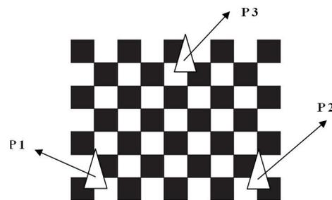
Figure 2: Three control points selected from the grids of the chessboard pattern.
