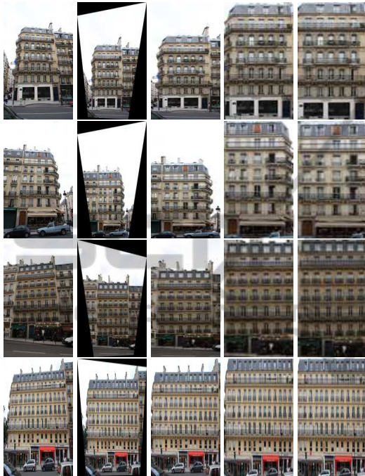
Figure 8: Results on Soufflot Street Facades. Left to right, original, rectified, cropped, final and ground truth.
