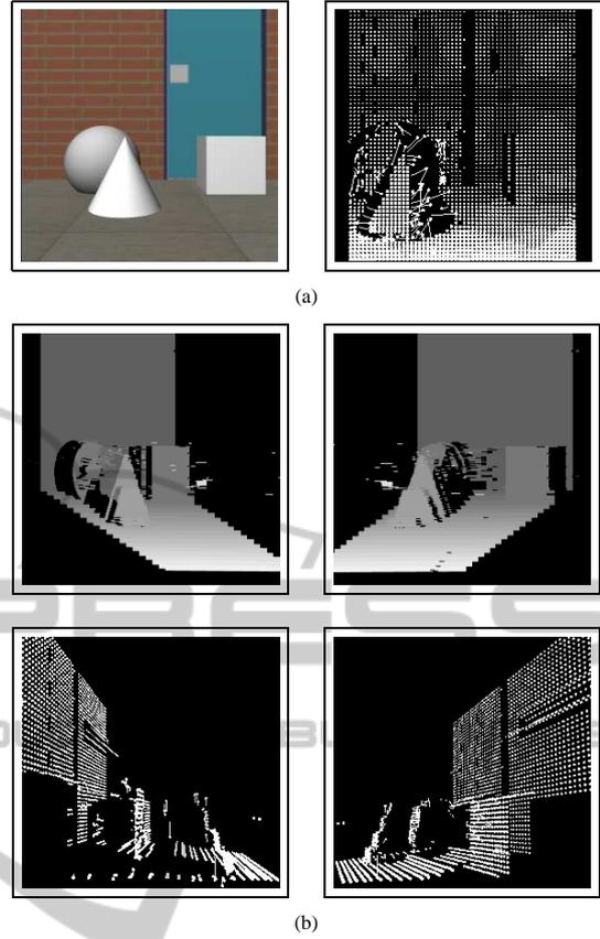
Figure 4: 3D Representation of MVFs generated from the simulated framework (Simore). (a) Left, an acquired image from the mounted stereo camera head in Simore. Right, the generated MVF. (b) Left, the spatial positioning error of direct 3D representation of disparity maps. Right, the result of the 3D MVF representation of the proposed approach.
