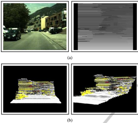
Figure 5: 3D Representation of MVFs generated from the DIPLODOC road stereo sequence. (a) Left, an acquired image from the mounted stereo camera. Right, the generated depth map. (b) The result of the 3D MVF representation of the proposed approach.
