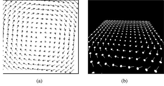
Figure 2: Rotation around  $z$  axis. (a) using the rotation parameter coefficient  $c_6$ , (b) perspective view of the transformed rotation parameter  $\theta_z$  using OpenGL.
