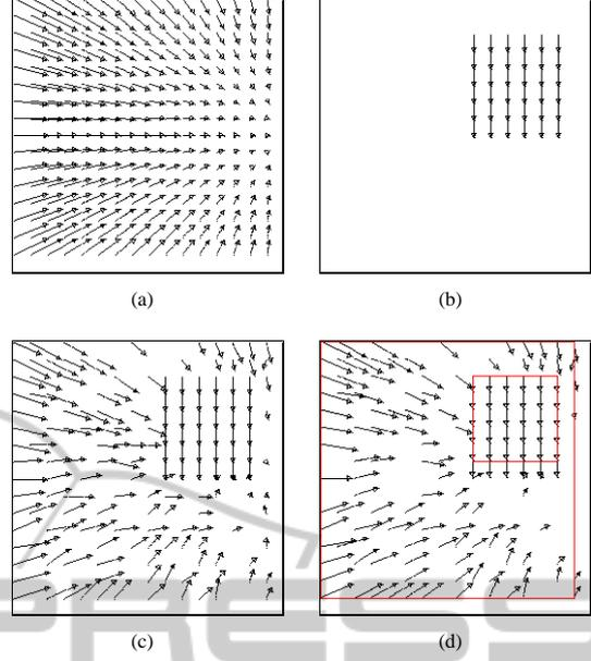
Figure 1: Segmentation of two different synthetic motions: (a) first motion, (b) second motion, (c) noisy MVF consists of the two previous motions, (d) result of the motion segmentation approach.
