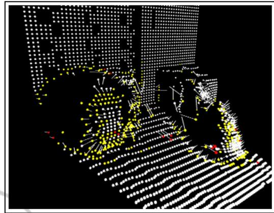
Figure 6: Detection of 3D motion patterns, yellow MVs represent the translation in the  $z$  direction which represents a possible collision with the robot.
