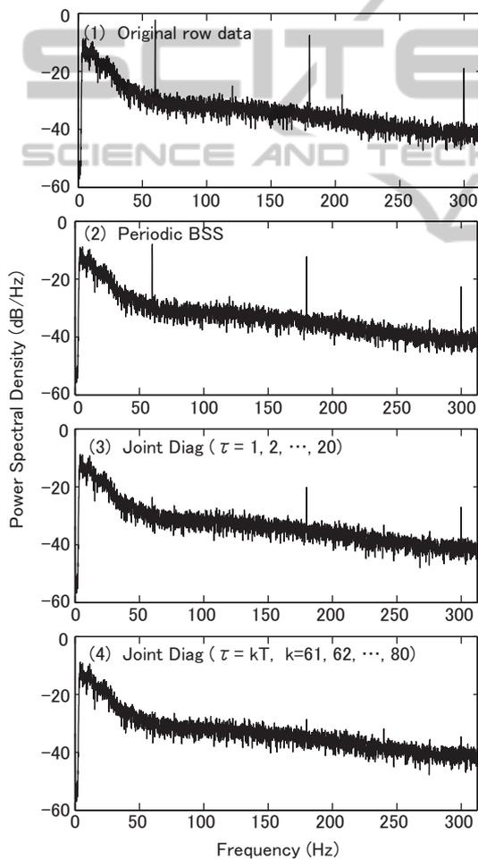
Figure 4: Power spectral density of MEG channel L42. (1) original row data, (2) after noise reduction using Periodic BSS, (3) after noise reduction using JADCM with conventional parameter set  $\tau = 1, 2, \dots, 20$ , and (4) after noise reduction using JADCM with proposed parameter set  $\tau = kT, k = 61, 62, \dots, 80$ .
