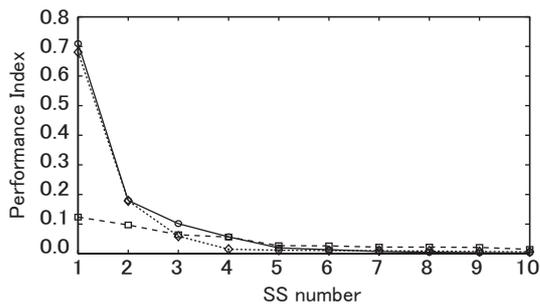
Figure 3: Performance indexes of SSs separated by Periodic BSS (dashed), JADCM with conventional parameter set  $\tau = 1, 2, \dots, 20$  (dotted), and by JADCM with proposed parameter set  $\tau = kT, k = 61, 62, \dots, 80$  (solid). The SSs are sorted according to the performance indexes.
