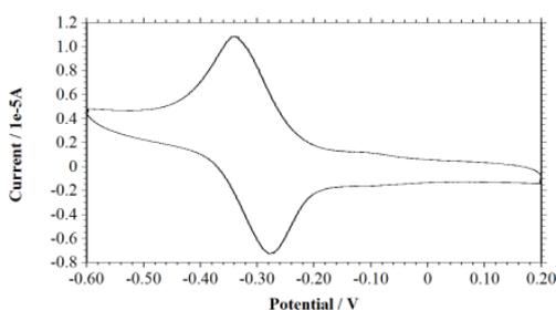
Figure 2: CV of methylene blue, Conc.: 100  $\mu\text{M}$ , in KCl 200 mM, scan rate 0.1 V/s.
