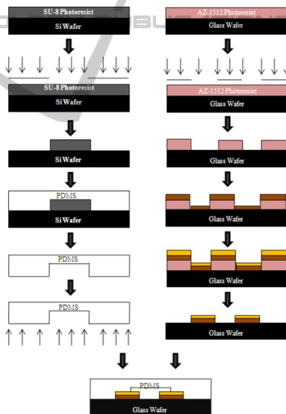
Figure 1: Fabrication of CE-AD device.
