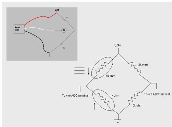
Figure 4: Design of load cells used in force platform.
