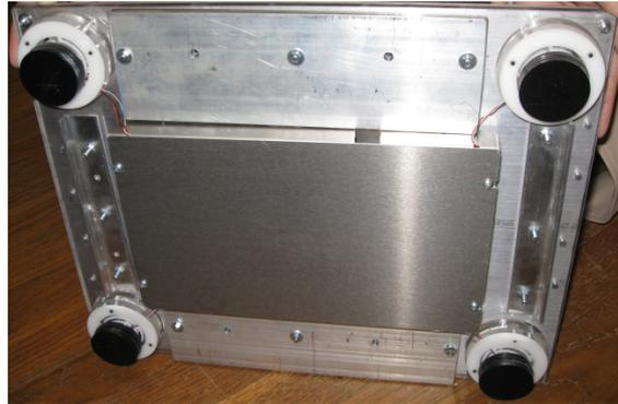
Figure 2: Bottom view of iBalance force platform.
