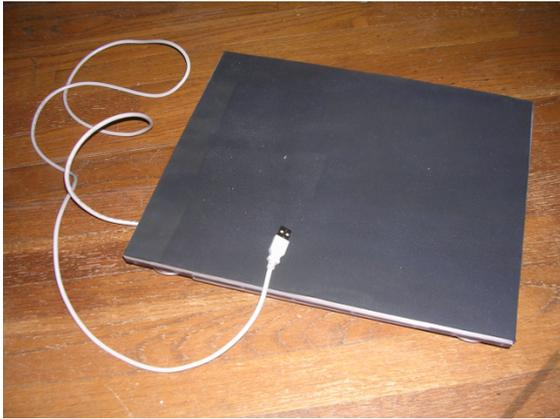
Figure 1: iBalance hardware consisting of a force platform with an USB extension chord for connection with an external computing device. The device has dimensions of 17" x 14" x .25" and weighs less than 10 lbs; substitution of lighter materials for the metal casing can significantly reduce the weight and increase the portability of the device.
