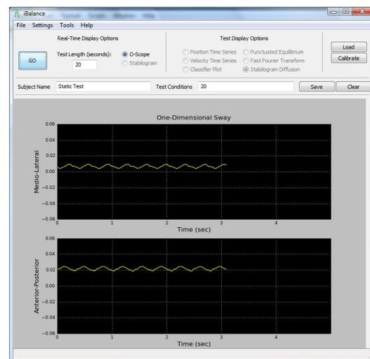
Figure 9: Oscilloscope view of real-time data collection from iBalance.
