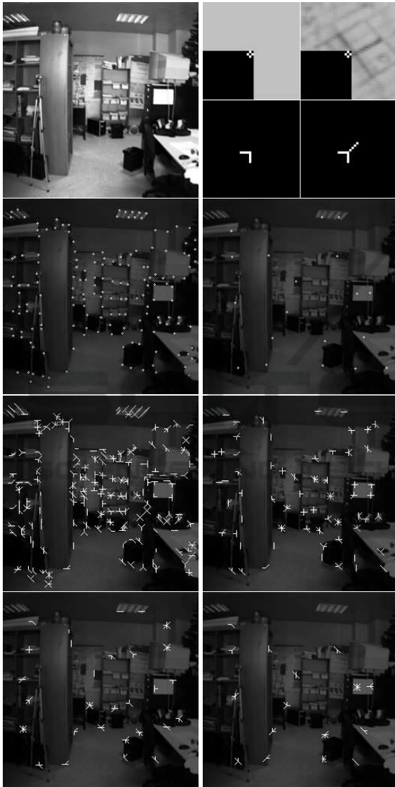
Figure 1: Keypoint detection and annotation. Input scene (top-left) with, on the 2nd row, keypoints detected at scales \lambda = 6 (left) and 27 (right). The 3rd and 4th rows show annotated keypoints at scales \lambda = \{6, 12, 18, 27\} . The top-right image shows one quadrant of a black square against a homogeneous background (left) and noisy background (right), both at \lambda = 6 .
