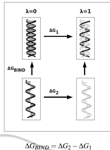
Figure 2: Thermodynamic cycle used in binding free energy calculations. The two branches of the cycle have to be considered in order to obtain the free energy of binding between the ligand, mRNA, and the receptor miRNA.
