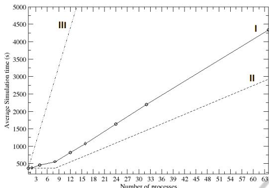
Figure 4: Trend of the simulation time at the increasing of the running processes. Trace 'I' and 'II' are respectively the real and the ideal trend for the simulation time obtained by running an increasing number of parallel processes, whereas trace 'III' is that relative to an increasing number of serial processes. The cycles on Trace 'I' mark the number of processes for which the test have been made.
