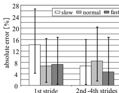
Figure 5: Evaluation results of stride length estimation. Average, minimum and maximum values of absolute error are shown for the 1st stride and from the 2nd strides.
