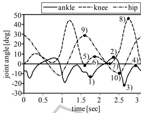
Figure 6: An Example of joint angles for two gait cycles. The numbers on the plots indicate the characteristic points which were analyzed in this paper.
