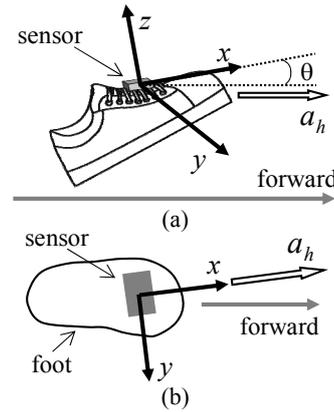
Figure 2: Attachment of sensors on the foot and velocity in forward direction. Side view (a) and top view (b).
