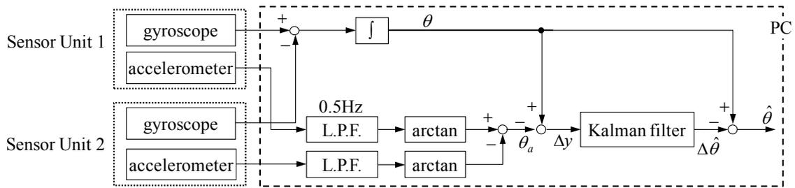
Figure 1: Block diagram of angle measurement system with Kalman filter.
