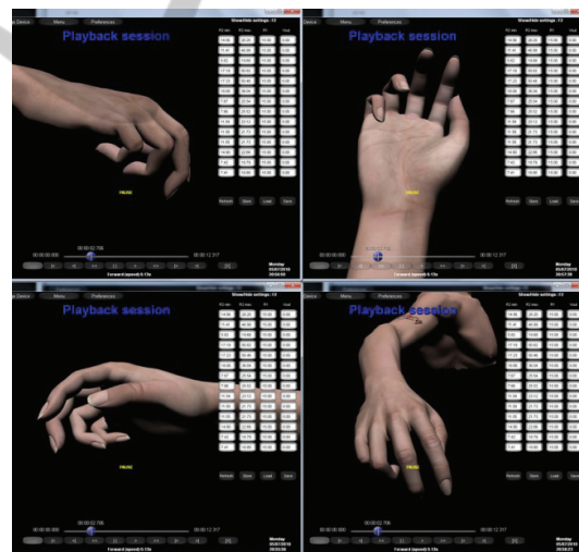
Figure 9: A reproduction session: software allows user to see an acquisition session off-line, and by rotating 3D model in any direction, it is possible to analyze reproduction from different viewpoints.
