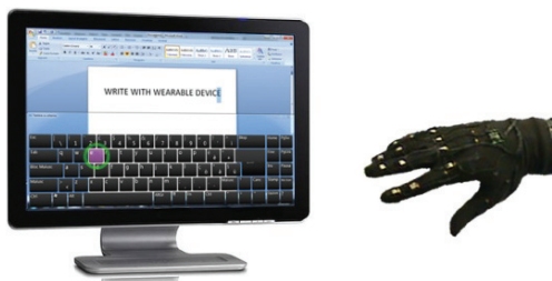
Figure 1: Data glove commands virtual keyboards.
