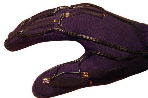
Figure 4: Lycra - based HITEG Glove.
