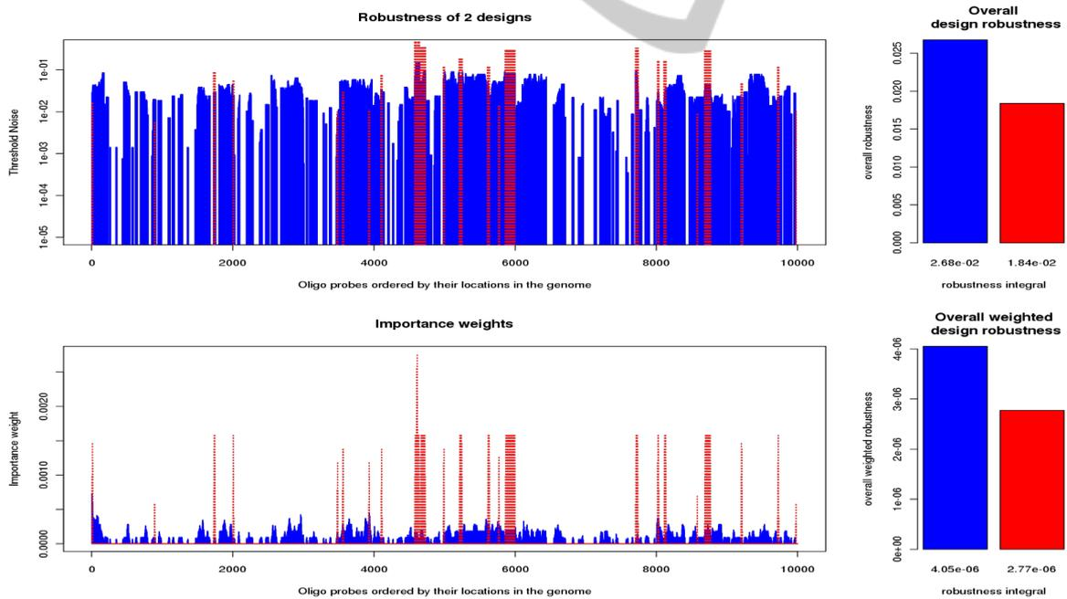
Figure 4: The robustness compared for two synthetic designs. The robustness has been calculated for all probes (upper plot) as well as corresponding weights importance (lower plot). The structure of genomic rearrangements mimics the abnormalities in classical genetic disorder (relatively rare long aberrant segments). Good design is coded in blue. Red design contains 15% of outliers (probes causing erroneous scanning).
