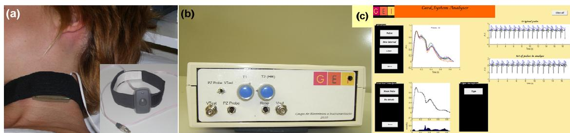
Figure 1: The main components of our non-invasive system for hemodynamic analysis. (a) PZ probe; (b) Acquisition box; (c) Graphical User Interface.
