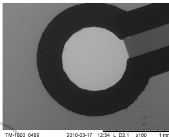
Figure 2: Electron microscope image of a working electrode of three-electrode structure (TES).
