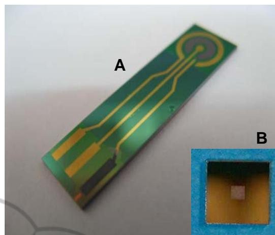
Figure 1: Silicon-based transducers used in this work: A – three-electrode structure (TES) (dimensions 7x26 mm); B – back-side contact structures (dimensions 5x5 mm).
