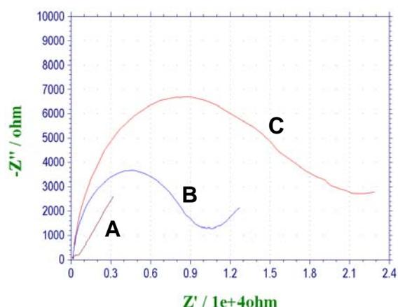
Figure 3: Impedance spectra of TES transducer with: A – bare gold electrode; B – DNA receptor layer; C – after hybridization.
