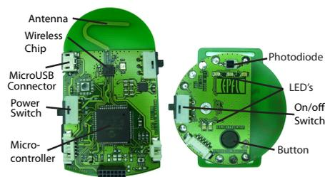
Figure 2: Bottom view of the *SleepPic Core* processing module (left). Top view of the *SleepPic Watch* module prototype (right).
