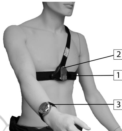
Figure 1: A subject wearing the complete SleePic sleep / wake detection system. 1) Equivalital™ Sensor Belt; 2) SleePic Core extension module; and 3) SleePic Watch for user interaction.
