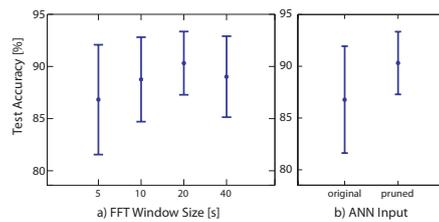
Figure 3: a) Performance analysis for different sliding window sizes (5, 10, 20 and 40 seconds) for the FFT preprocessing. b) Performance comparison when the entire feature set (original) or the reduced feature set (pruned) is used as input of the ANN. The bullets represent the mean over all trials and subjects, the bars cover the standard deviation.
