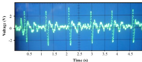
Figure 4: ECG signal obtained at the end of the first circuit module. The average amplitude of the signal is 3 V.
