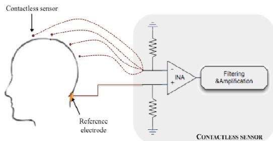
Figure 1: Contactless sensor for biopotential acquisition. Dashed lines are used to indicate that the sensor may be placed in several recording locations.
