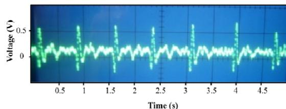
Figure 6: ECG signal recorded at a distance of 1cm from the INA116. An isolated probe was used to carry the signal from the first module. The average amplitude is 600 mV.
