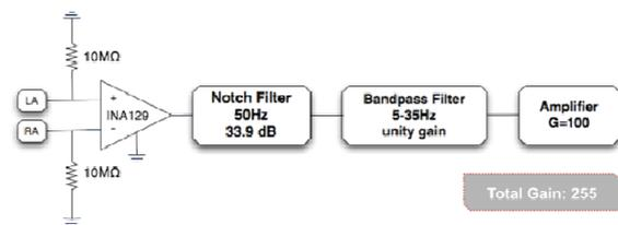
Figure 2: First module comprising a conventional acquisition circuit for biopotentials. LA corresponds to Left Arm, and RA to right arm.
